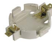
BU2032SM-JJ-MINI-GTR recessed into pcb
