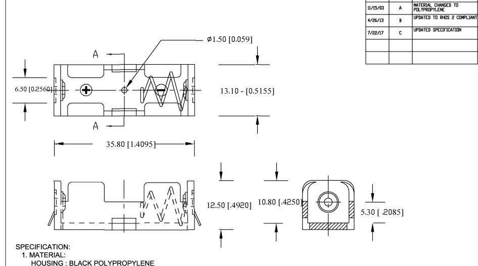
SOLDER LUG: STEEL, NICKEL PLATED. SPRING: SPRING STEEL, NICKEL PLATED LUGS: BRASS, NICKEL PLATED CONTACT RESISTANCE: UNDER  $50m\Omega$  FOR +/- CONTACTS PER EIA-540J000 **ROHS 2 COMPLIANT**
